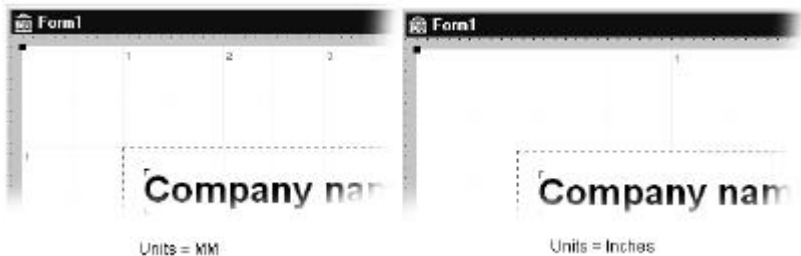
Figure 6 - Adjusting the Units property to alter grid spacing
